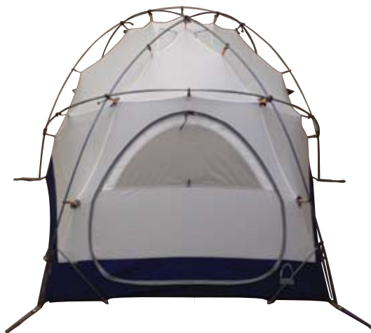
Clip-Loc™ attachment-wrap bungee around pole twice and lock in slot
